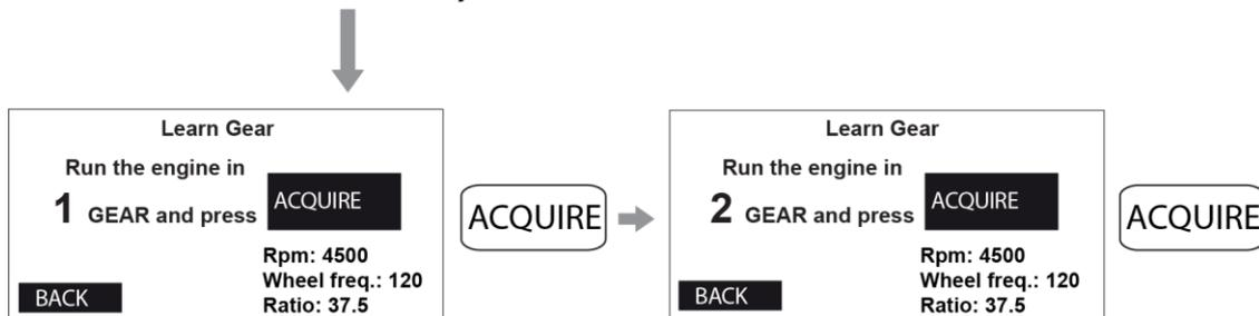
Please Note: Since the gear must be as stable as possible during the learning cycle on the stand, it is recommended to press the rear brake slightly during storage so as to reduce drive oscillations to a minimum.
