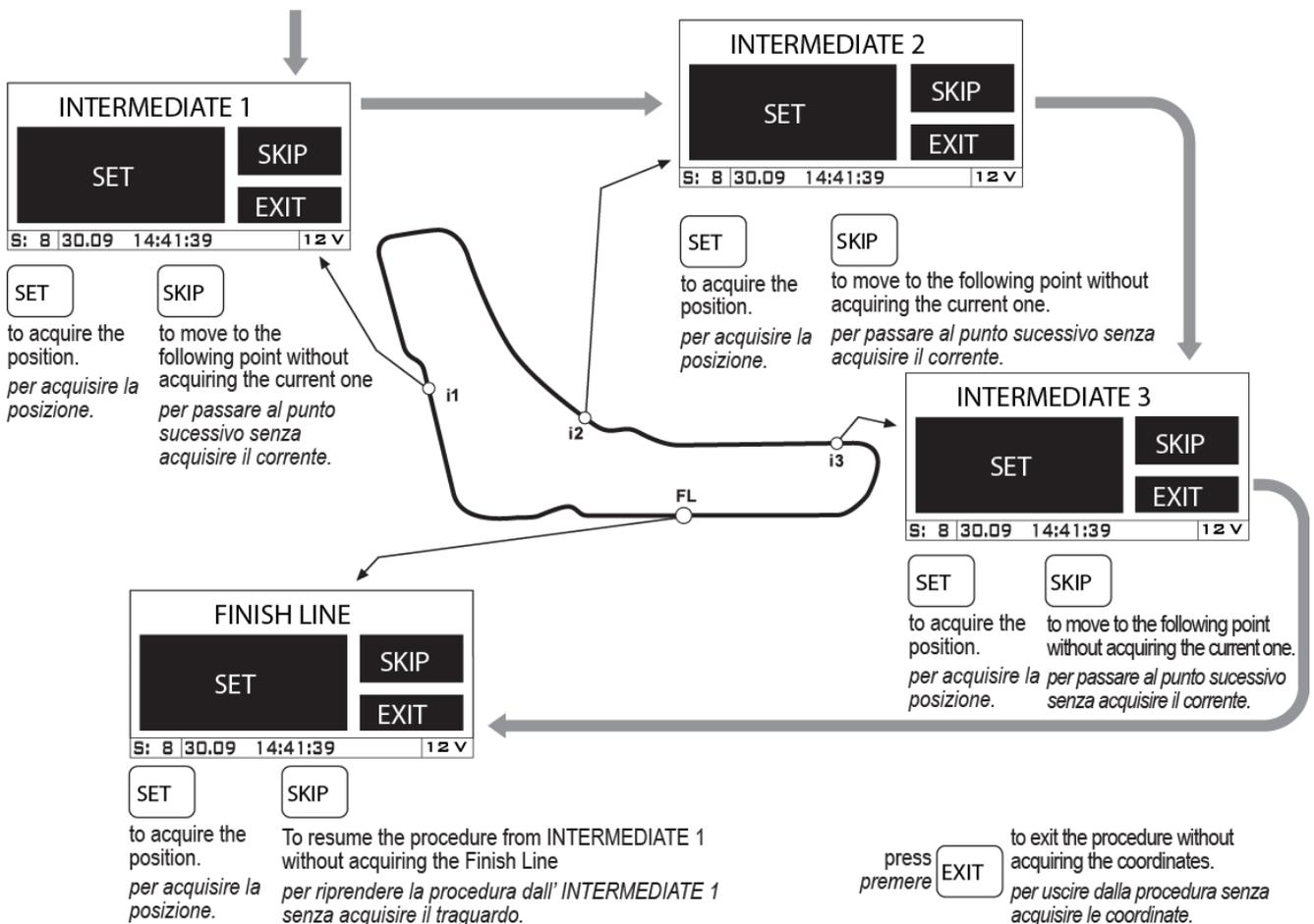
Every time the **SET** button is pressed the Best LED will flash white (to confirm the button has been pressed) immediately followed by a Green flash if the coordinates are correct or Red if GPS signal was missing.
