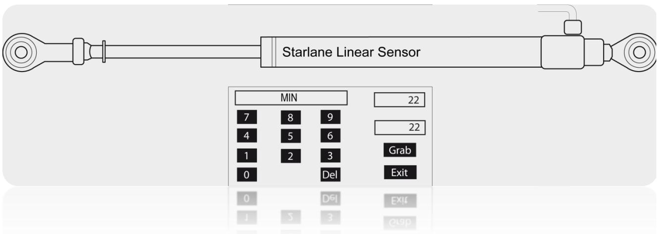
5. Close the sensor completely so as to move the Seeger to the stroke limit.
