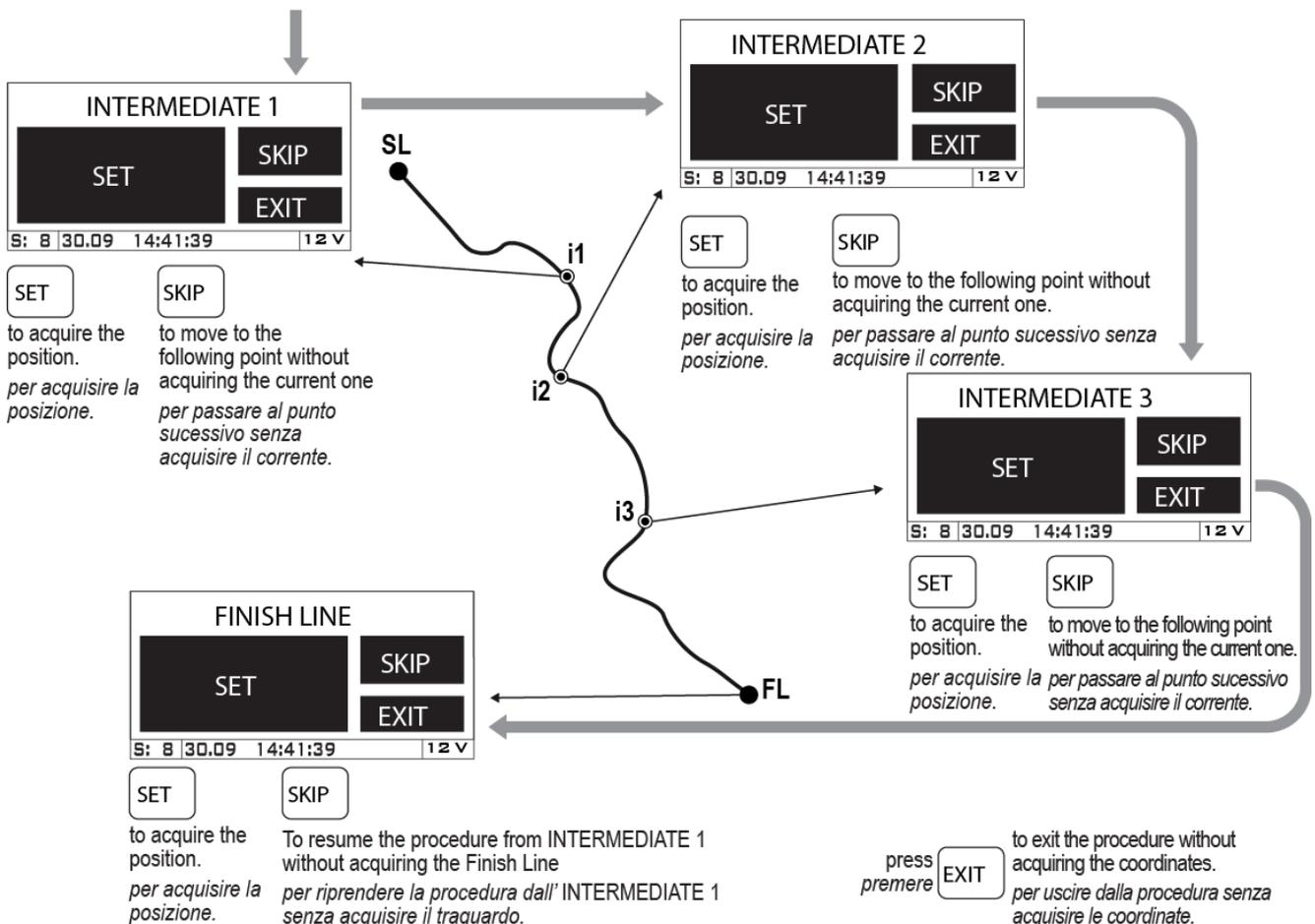
NOTA: you are not required to set up the Start Line in the still start mode since the device starts timing when the internal accelerometer detects the movement upon the vehicle start-up.
