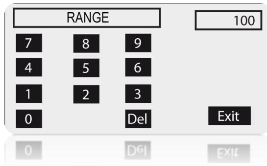
Digit **100** on the keyboard (you can delete existing values using the <- key) and press **EXIT** to exit.
