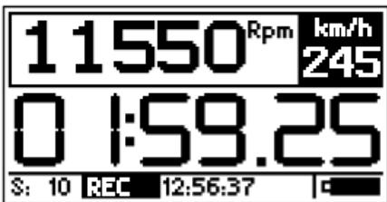
While **CORSARO-II** is recording the REC label blinks at the bottom of the screen.
