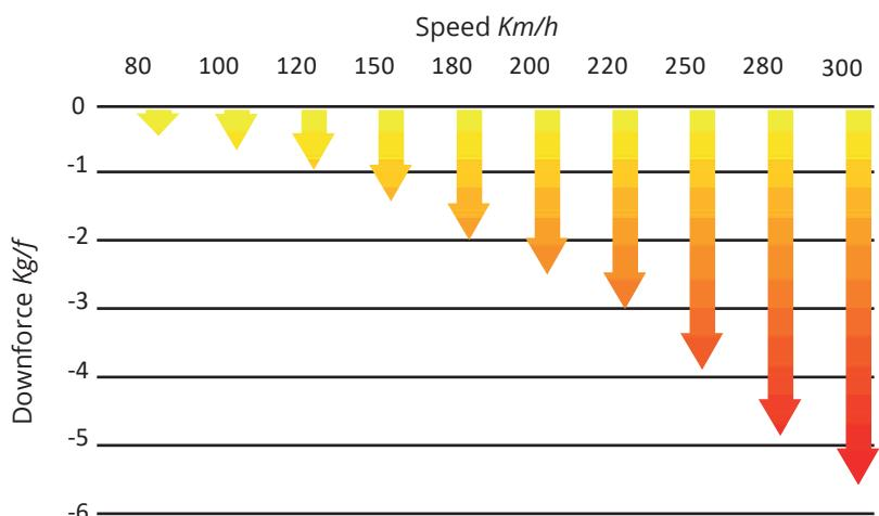
The Downforce that the spoilers generates raises potentially as the speed increases, at 300 km/h we get 5.6 Kg/f.
