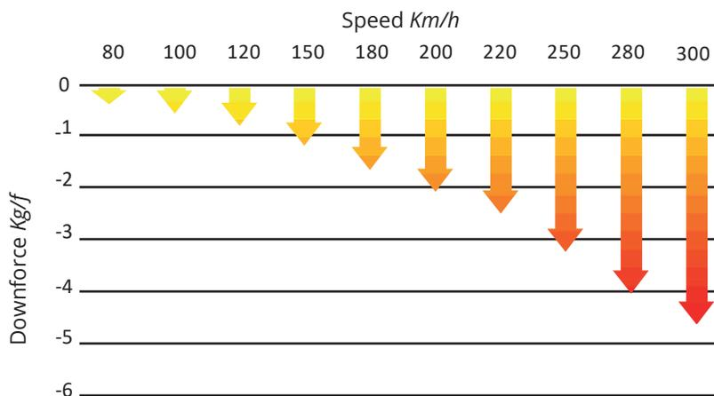
The Downforce that the spoilers generates raises potentially as the speed increases, at 300 km/h we get 4,6 Kg/f.
