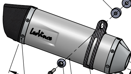
Aluminium spacer ø30X15x8.5 Cod. 206663
