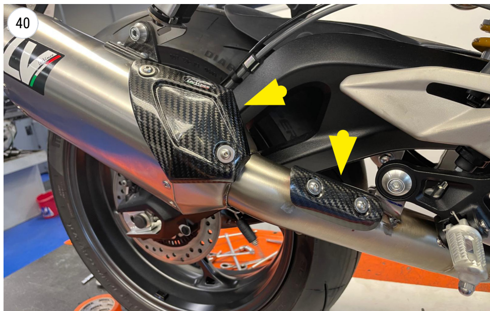
FIT THE CARBON HEAT SHIELDS
