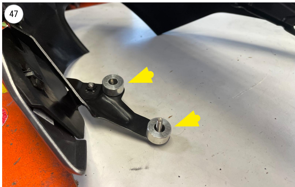
FIT THE SPACER ON THE LOWER FAIRING
