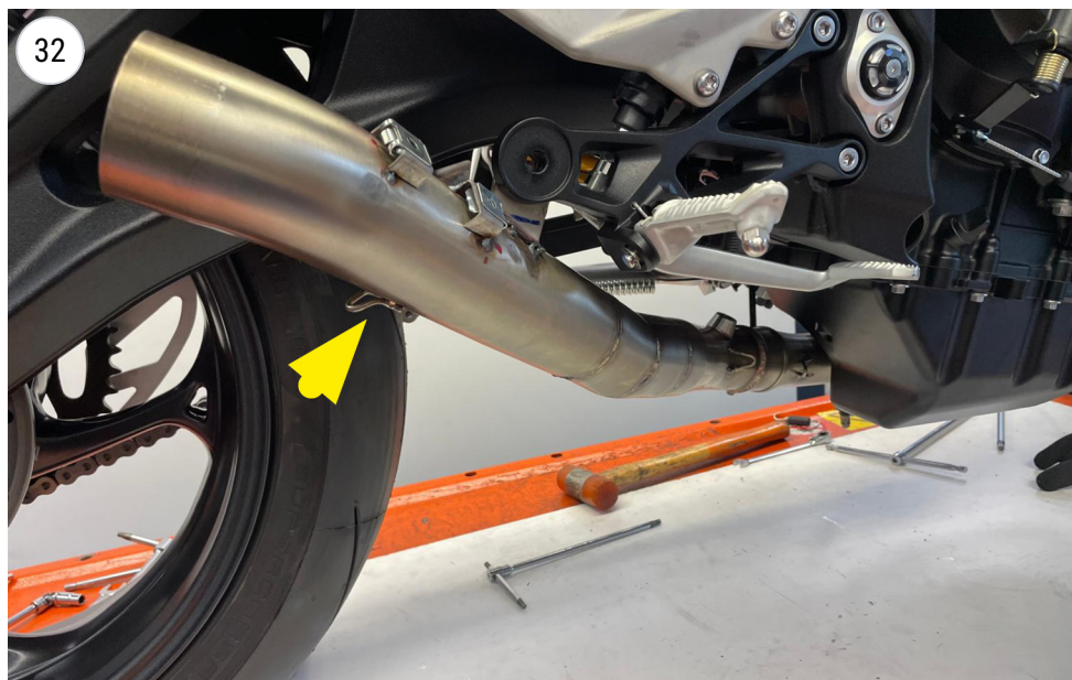
FIT THE FINAL LEOVINCE PIPE
