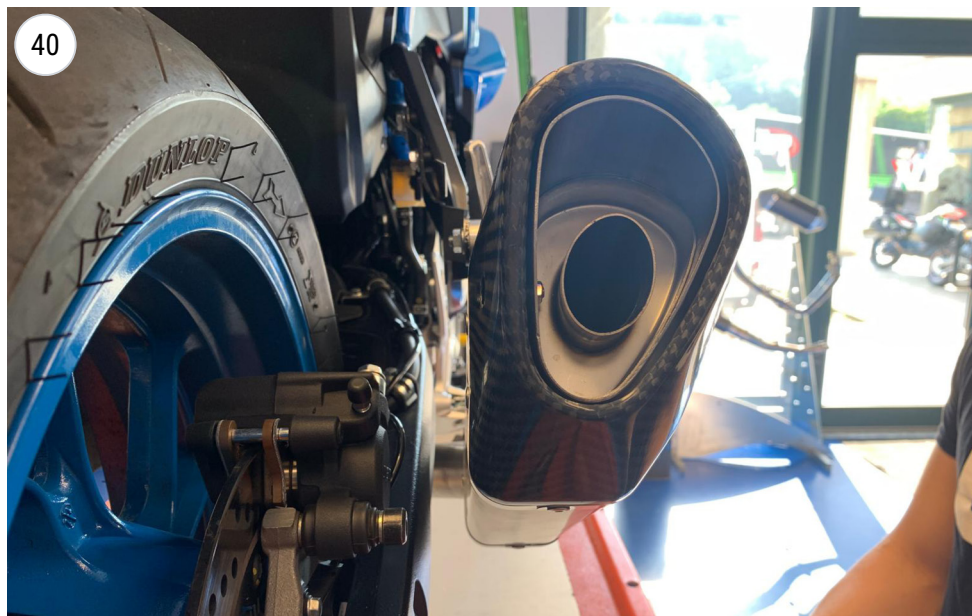
CHECK THE POSITION OF THE MUFFLER
