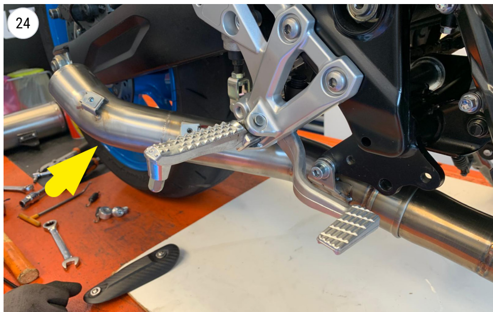
INSTALL THE FINAL PIPE
