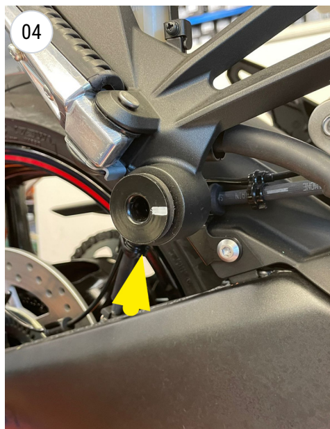
REMOVE THE STOCK SPACERS
