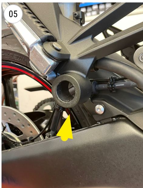
REMOVE THE STOCK SPACERS
