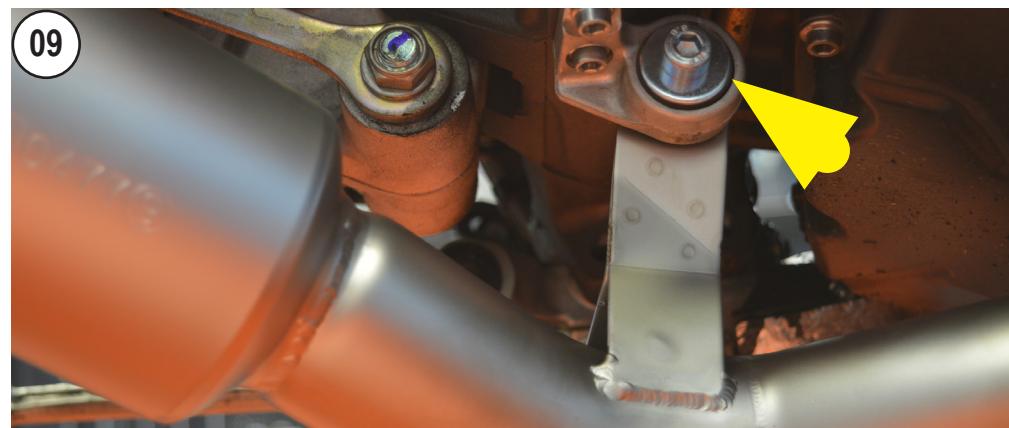
FIX THE BRACKET TO THE FRAME
