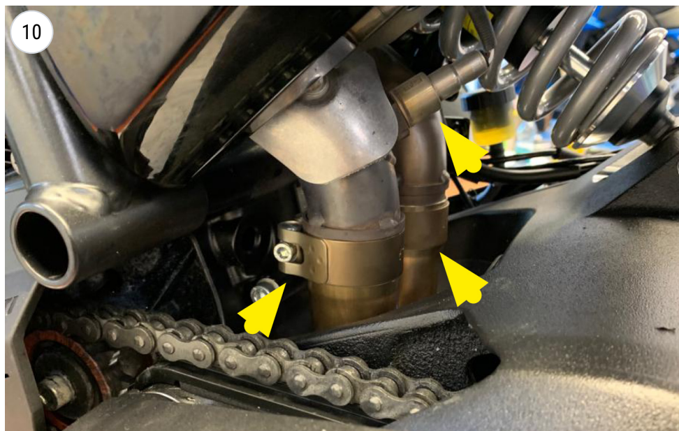
tight the clamp and screw the sonda lambda/O2 sensor
