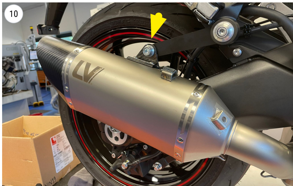
FIT THE MUFFLER AND SCREW - MOUNTING FOR KAWASAKI NINJA 1000/1100 SX
