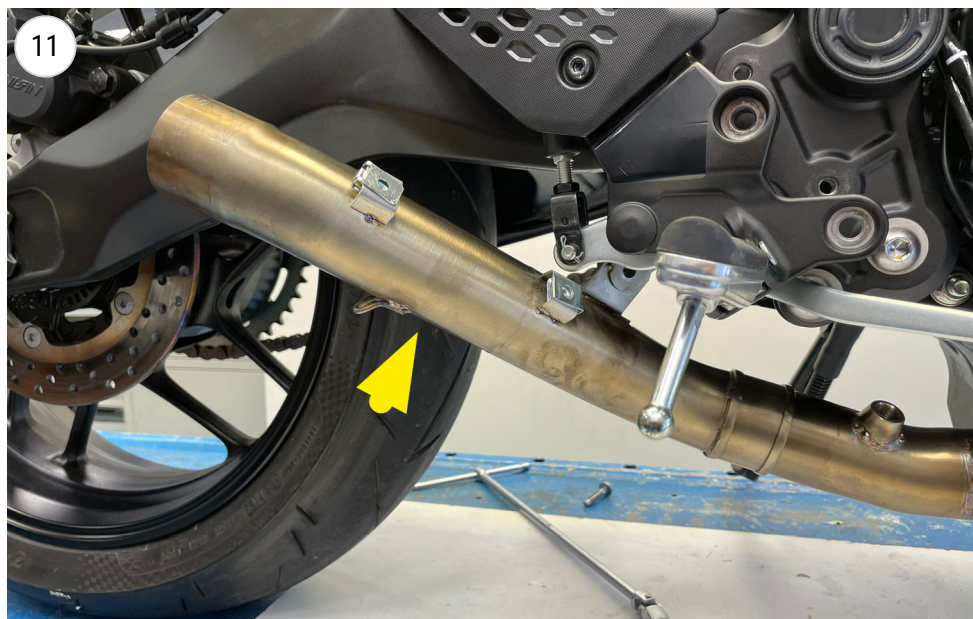
fit the final pipe
