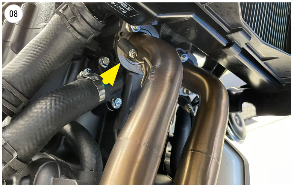
Fit the primary pipes
