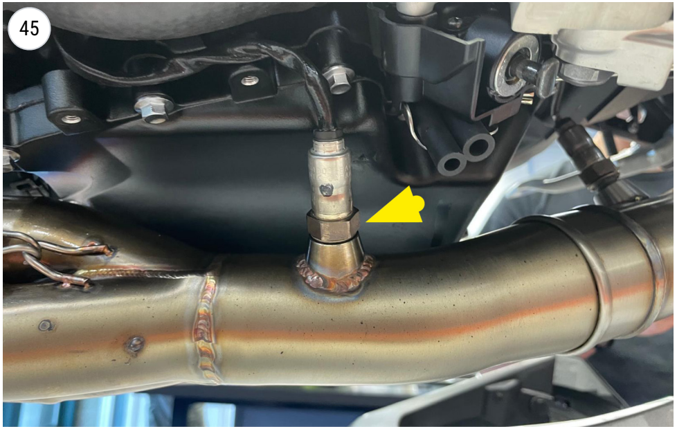
SCREW THE OXYGEN/LAMBDA
