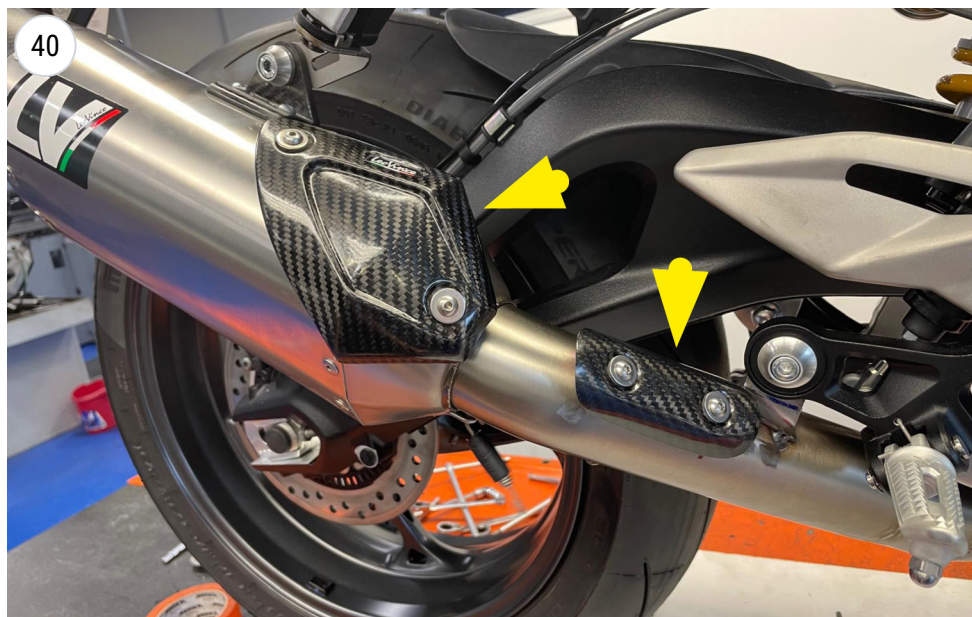
FIT THE CARBON HEAT SHIELDS
