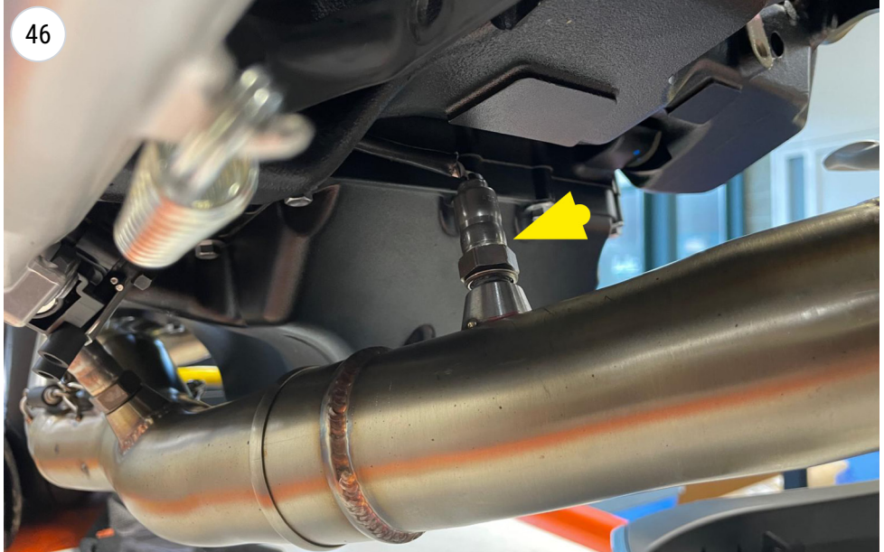
SCREW THE OXYGEN/LAMBDA
