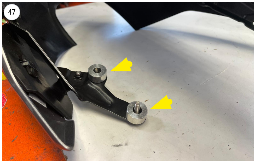
FIT THE SPACER ON THE LOWER FAIRING
