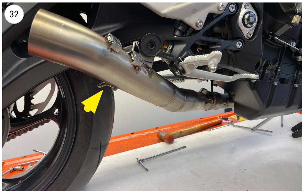
FIT THE FINAL LEOVINCE PIPE
