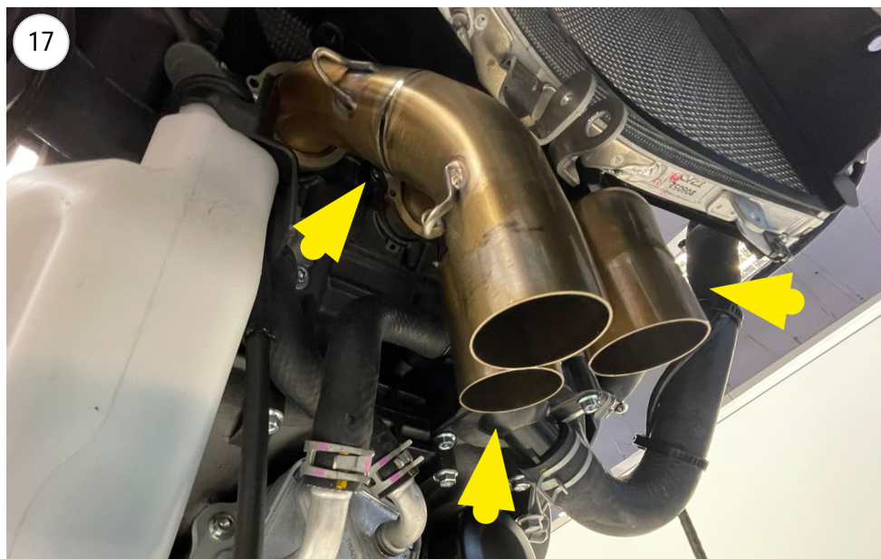
fit the primary pipe
