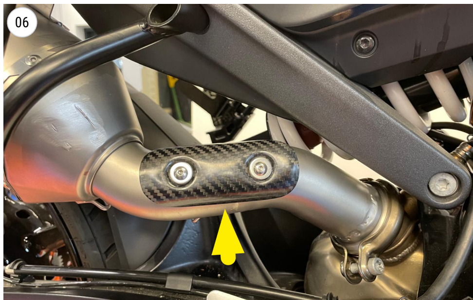
fit the carbon heat shield
