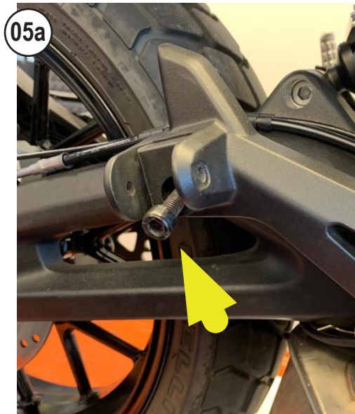
REMOVE THE SCREW AND THE FOOTPEG
