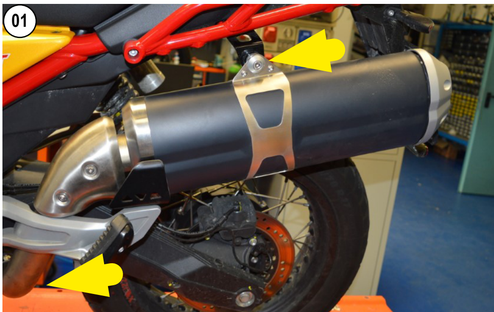
LOOSE THE CLAMP, UNSCREW AND REMOVE THE STOCK MUFFLER
