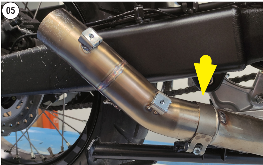
SLIDE THE PIPE IN WITH THE CLAMP
