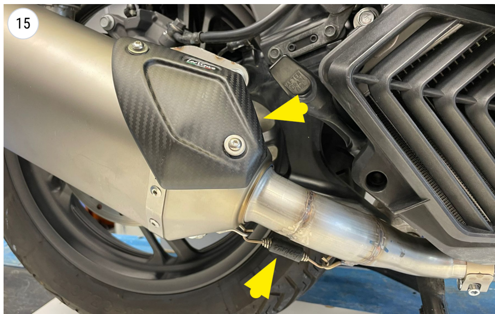
fit the carbon heat shield and hang the spring
