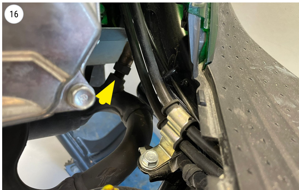
screw the Sonda lambda / O2 Sensor
