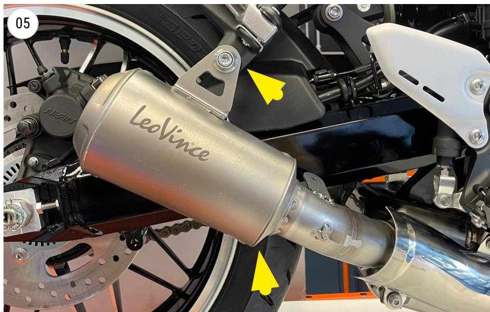
install the muffler with the clamp
