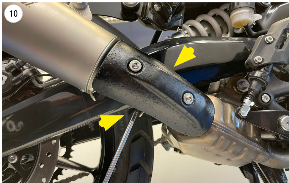
fit the carbon heat shield, align it and tight the clamp
